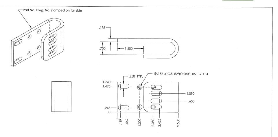
MATERIAL: ALUMINUM 5052-H32 FINISH: TIME SAVED, DEEP BLUE ANODIZED (15 MIN. IN BLUE DIE)
