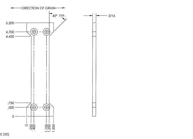
MATERIAL: ALUMINUM 5052-H32 THICKNESS: 3/16" FINISH: TIME SAVED, DARK BLUE ANODIZED (15 MIN. IN BLUE DIE)
